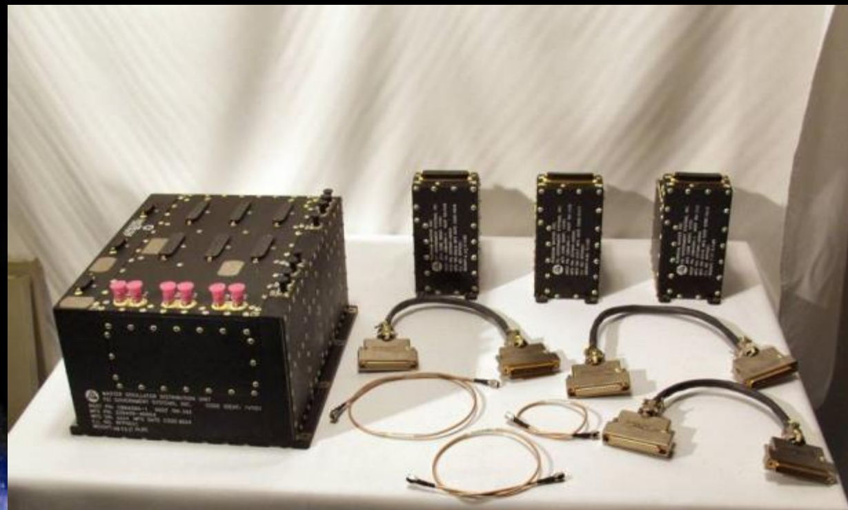
AEHF Master Oscillator Group (MOG) - 3 Redundant Rb Master Oscillators
