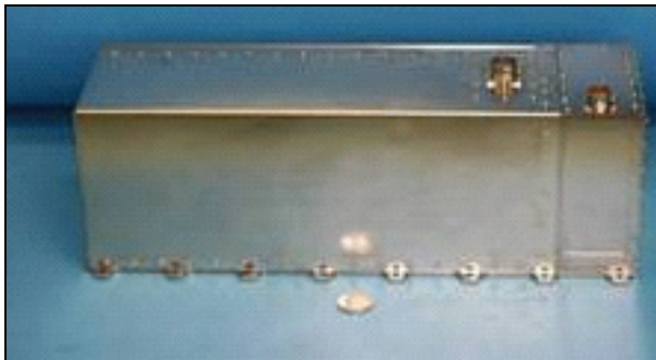
Rubidium atomic timing system for GPS III- FEI's highest precision frequency standard for space
