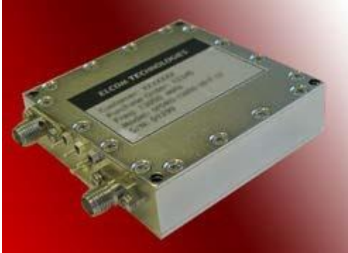
Ultra-Low Phase Noise, Multiple Frequency Options, Low Spurious, Size: 2.25" x 2.25"x 0.65"
